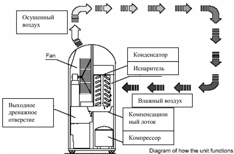
Diagram of how the unit functions
